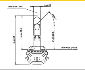
Light center length: 31,75mm ± 0,5mm Bulb diameter: max. 9mm
